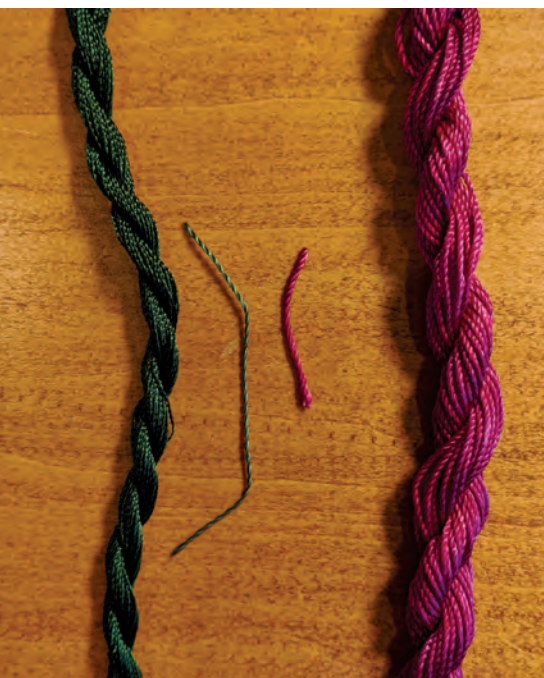
Z-twist on the left and S-Twist on the right
